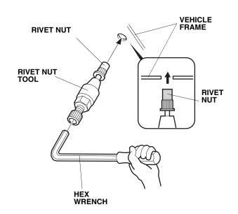
• While holding the rivet nut tool with the hex wrench, use a 27 mm wrench to turn the tool clockwise to install the rivet nut into the hole in the vehicle frame.
